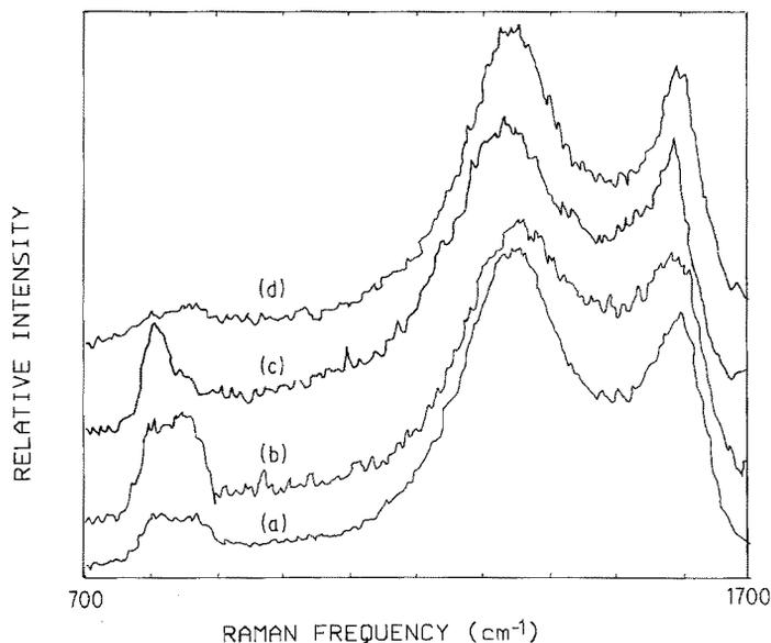
Figure 3 Raman spectra of silicon carbide fibres taken at increasing depths into the fibres: (a)  $0\text{ }\mu\text{m}$ , (b)  $0.2\text{ }\mu\text{m}$ , (c)  $0.9\text{ }\mu\text{m}$ , (d)  $3.8\text{ }\mu\text{m}$ .
