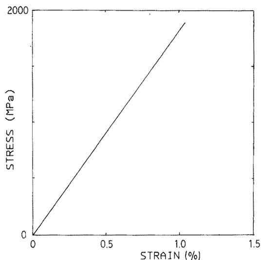
Figure 5 Typical stress-strain curve obtained for a single silicon carbide fibre.
