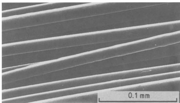
Figure 1 Scanning electron micrograph of the silicon carbide fibres.
