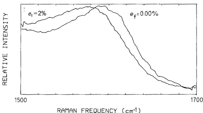
Figure 6 Detail of Raman spectra obtained from an unstrained fibre and the same fibre strained to 2% elongation.
