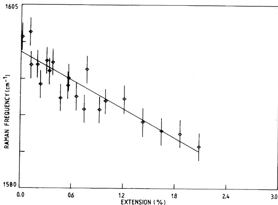
Figure 7 Variation of the  $1601\text{ cm}^{-1}$  Raman band with strain for several fibres.
