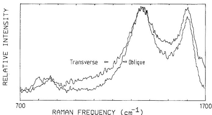
Figure 2 Raman spectra of a silicon carbide fibre taken at the centre of a transverse section and at the centre of an oblique section angled at  $18^\circ$  to the fibre axis.
