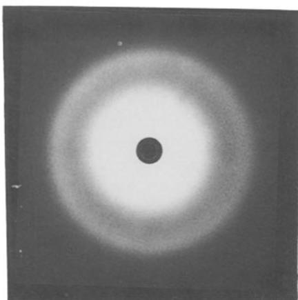
Figure 4 Wide-angle X-ray scattering pattern obtained from silicon carbide fibres.
